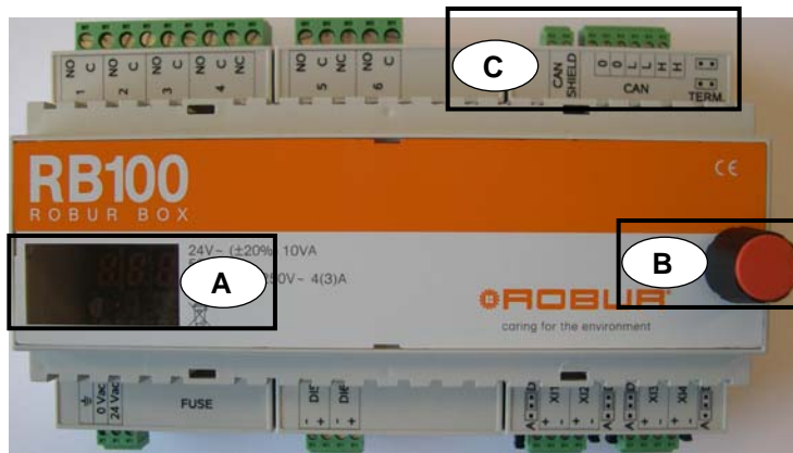
Figure 29 Complete RB100 interface. Display, Encoder and CAN-BUS port are pointed out.
