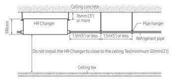
9. Select a place with enough space for repairing and services. (Leave enough space between sidewalls in installation.-refer to the picture below)
