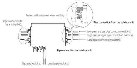
When installing HR Changer, use the pattern sheet for installation that is provided with the product. When welding the gas pipes, protect the product with the flame-proof sheet.
